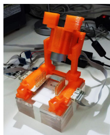
DMF platform for droplet control and impedance variation tests.
