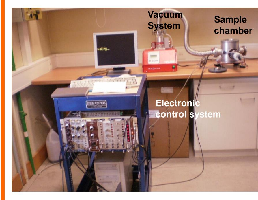
Thick Source Alpha Counting (TSAC) spectrometry technique using a silicon detector for <sup>226</sup>Ra and <sup>230</sup>Th quantification
