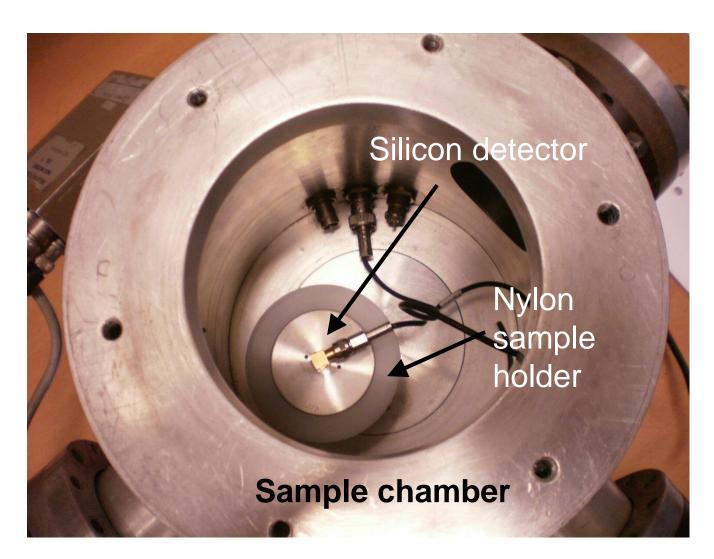
Ideal samples should be pressed forming pellets. For the measurements of  $\alpha$  particles emitted by these samples, a 1200 mm<sup>2</sup> silicon detector with a resolution of 32 keV is placed at around 5 mm from the sample in vacuum conditions (P=1.4×10<sup>-6</sup> mbar). The silicon detector is energy calibrated with a triple-alpha source (<sup>244</sup>Cm, <sup>241</sup>Am and <sup>240</sup>Pu).
