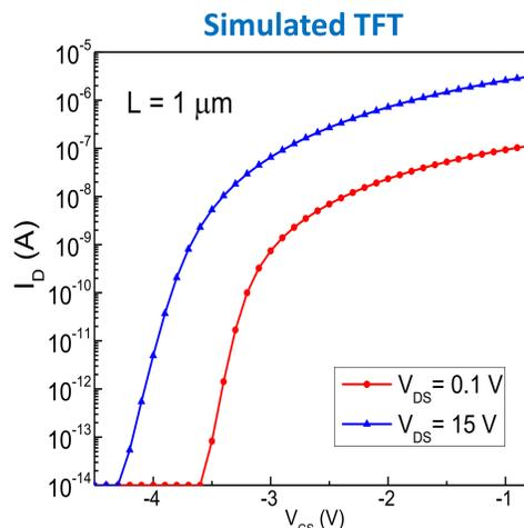
Simulation of a dual-gate TFT showing the effect of different biasing conditions for the second-gate.
