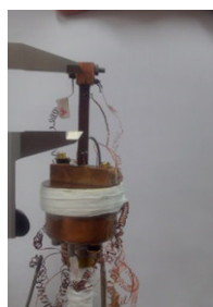
Thermal conductivity Measurements (3 K- 100 K)
