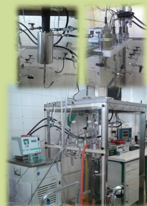
Gravimetric apparatus for adsorption equilibrium determination
