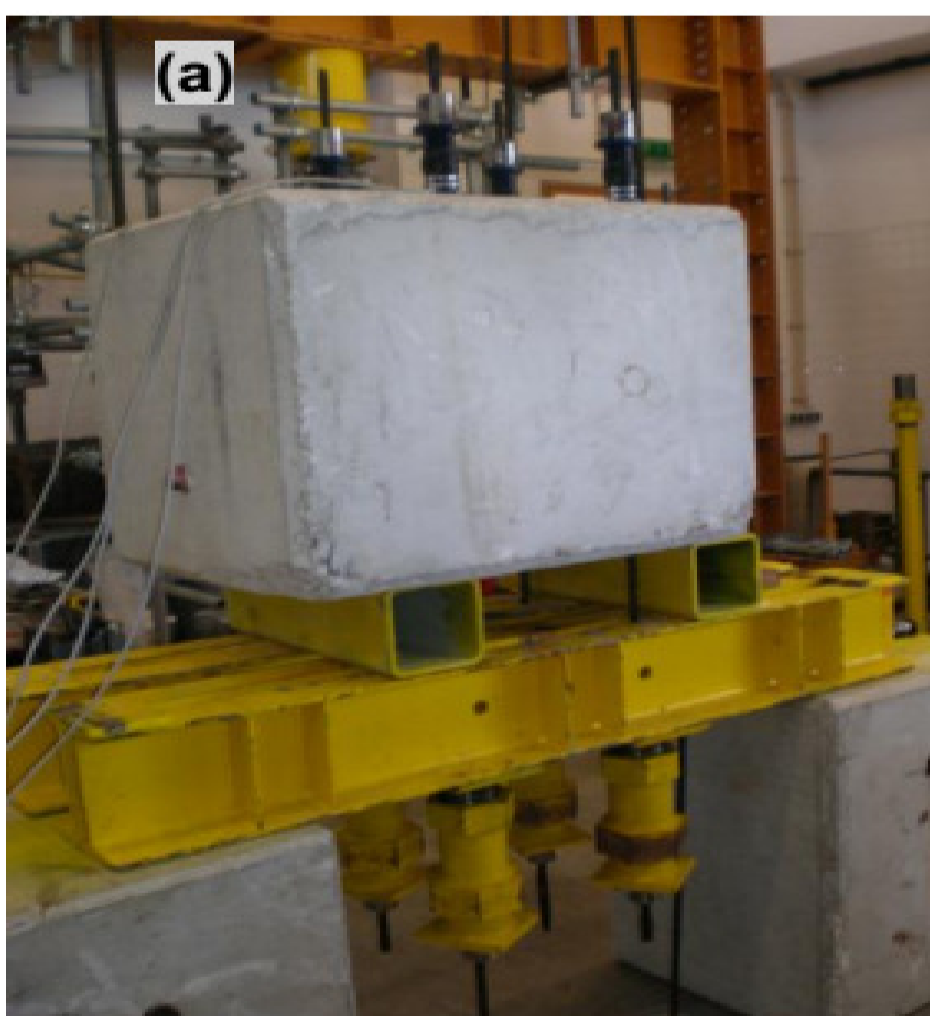
Fig.4: Set-up of long-term bond test (By Faria,V 2011)
