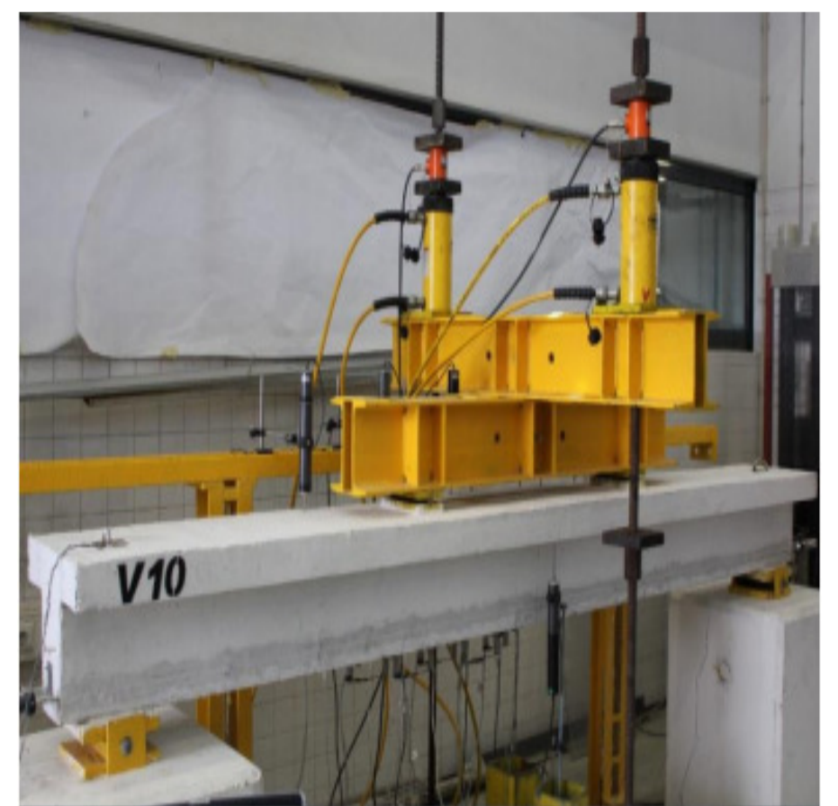
Fig.3: Set-up, test of RC Beam (By Monteiro, A 2014)
