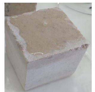
Fig. 2: Biotreated surface of a sample
