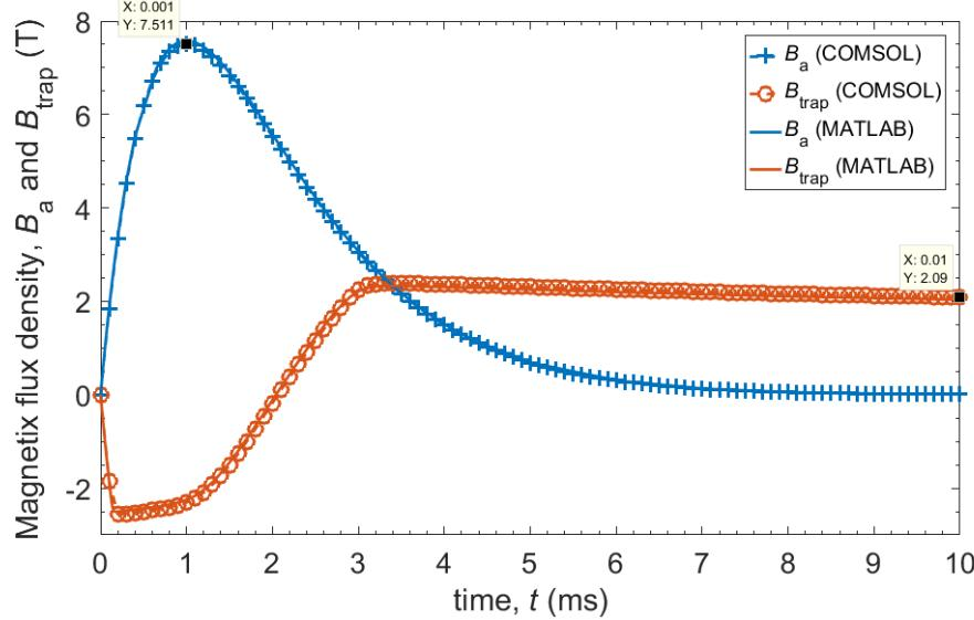
Applied magnetic field  $B_a$  and trapped magnetic field  $B_{trap}$  on the top surface of the bulk HTS, at  $r = 0$  and  $z = Z_{33}$ .
