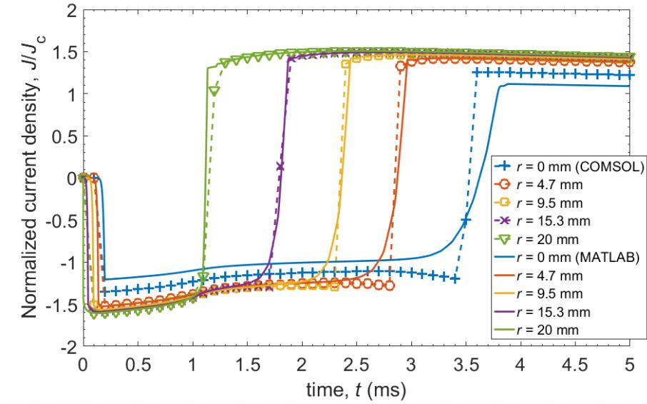
Normalized current density  $J / J_c$  in the middle plane of the bulk HTS for  $r = \{0, 4.7, 9.5, 15.3, 20\}$  mm.
