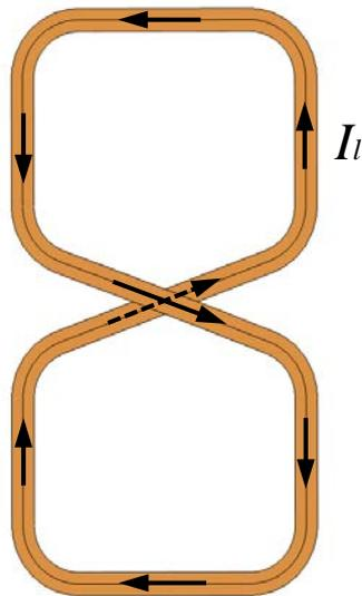
The direction of current in levitation coil
