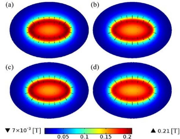
Distribution of magnetic field generated by a race-track magnet, (a) Simulation, (b) Line current, (c) Surface current, (d) Volume current
