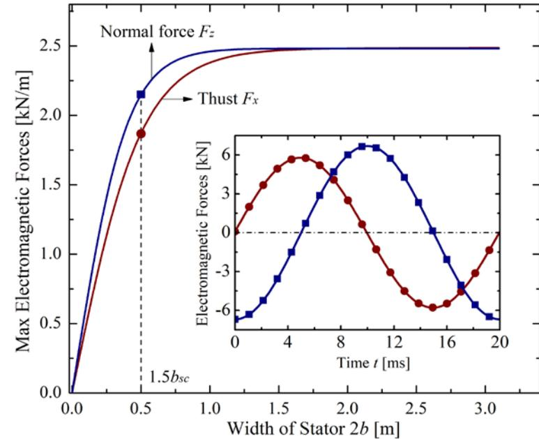
The thrust curve using optimized parameter
