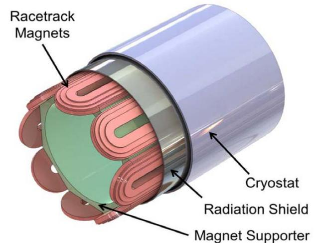
Design optimization for the HTS magnet of an HTS generator
