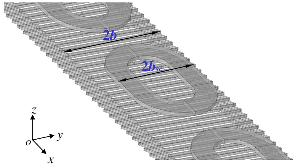
Geometric structure of air-core linear motor
