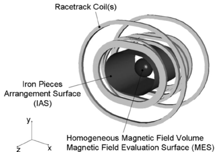
Design optimization for the racetrack HTS magnet construction
