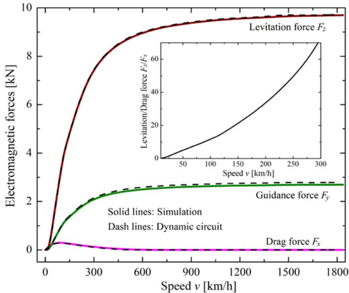
Maximum electromagnetic forces versus  $v$
