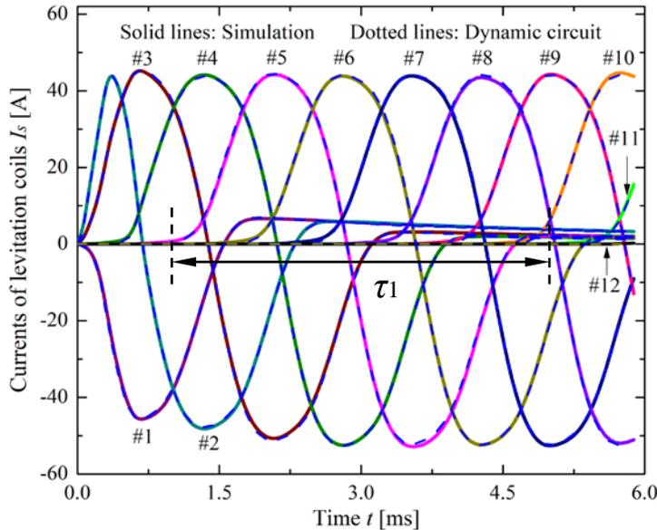
The induce current in levitation coils
