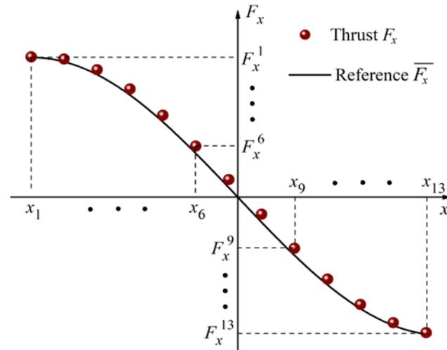
The thrust  $F_x$  of air-core linear motor
