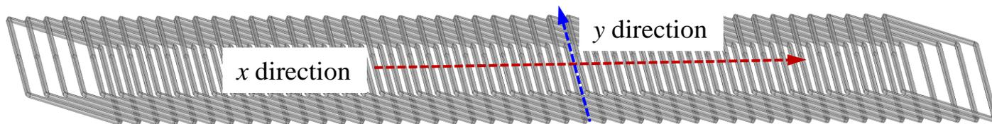
The geometric structure of a flat air-core stator windings
