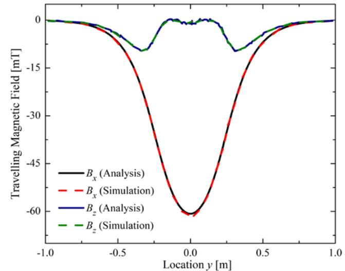
The travelling magnetic field generated by a flat air-core stator, including the horizontal component  $B_x$  and vertical component  $B_z$
