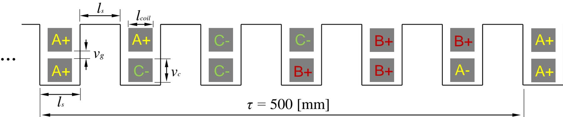
The geometric structure of air-core stator with double-layer copper windings
