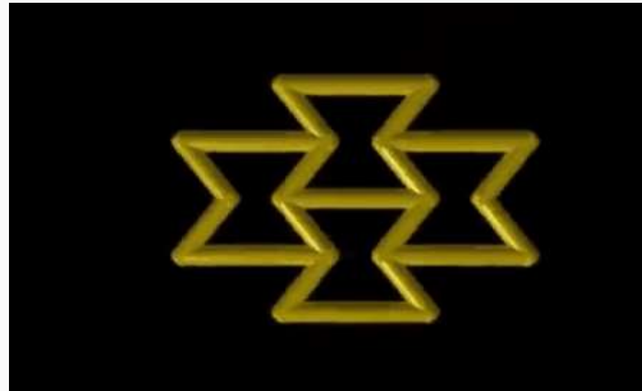
Animation of the behaviour of an auxetic material when undergoing uni-axial tension
