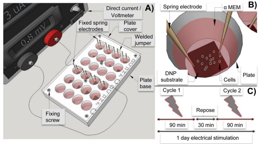
Schematic representation of the DC electrical stimulation apparatus
