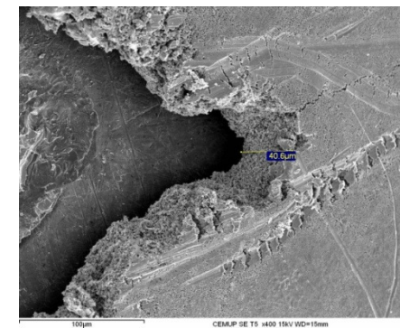
Aspect of the Ag membrane fracture
